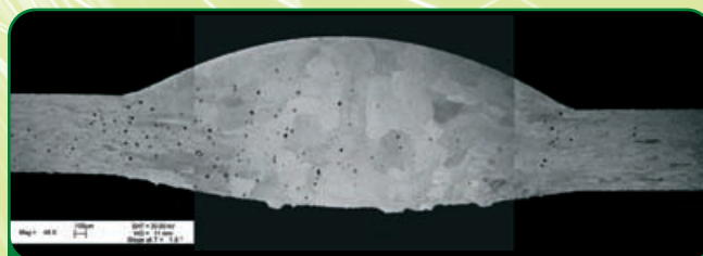
Fig. 3. Macrograph of a TIG weld. Very differently oriented and shaped grains are present together with cavities. Courtesy of O.Fraboulet (Corning SAS, CETC, Avon, France).
