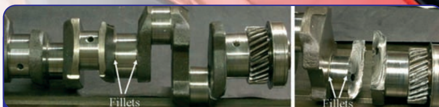
Fig. 1. Original and broken crankshaft. Failure was initiated at a fillet and propagated by fatigue
