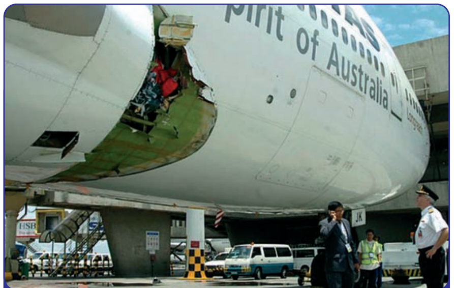
Fig. 2. Failure of a riveted aluminium skin panel which has penetrated the fuselage.
