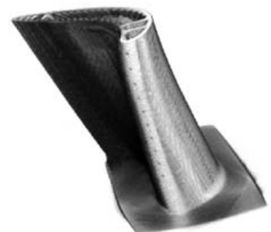
Fig. 4: Neutron tomographic reconstruction of a section of a coated Ni superalloy single crystal jet turbine blade.
